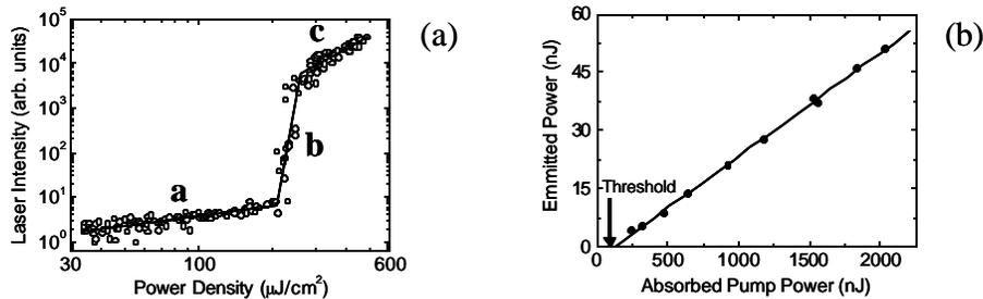
Fig. 3. (a) The laser emission intensity plotted against the pump intensity, where the lines are power law fits for each of the region referred as (a), (b) and (c) (see text for details). (b) Emitted laser power plotted against the absorbed pump power, the solid line being a linear fit with slope 0.027.
