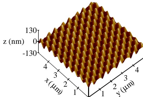
Fig. 1. AFM surface profile of DFB laser sample with three multiplexed gratings. The grating modulation depth is ~40 nm.
