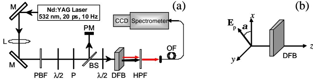
Fig. 2. (a) Experimental apparatus. M: mirror, L: lens, PBF: pass band filter, P: polarizer, BS: beam splitter,  $\lambda/2$ : half wave plate, DFB: distributed feedback laser sample, HPF: high pass filter, OF: optical fiber, PM : Power Meter (b) Orientation of the pump polarization direction impinging on the sample where  $\alpha$  is the angle between the pump electric field  $\mathbf{E}_p$  and the  $x$ -axis.
