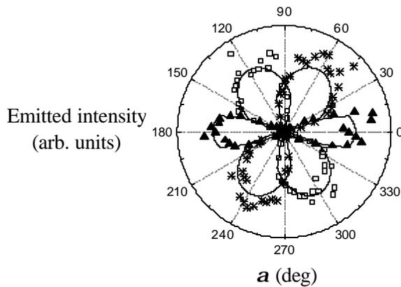
Fig. 5. The pump polarization dependence of the emitted laser intensity corresponding to the three multiplexed gratings. Open squares: peak at 630.6 nm, stars: 635.0 nm, filled triangles: 638.7 nm. Theoretical fits are described in text.
